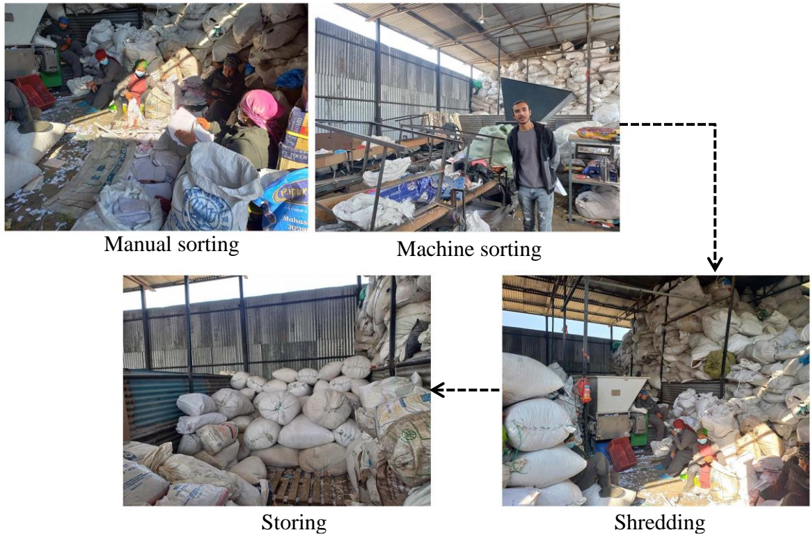
Figure 3. 19 Paper recovery process
