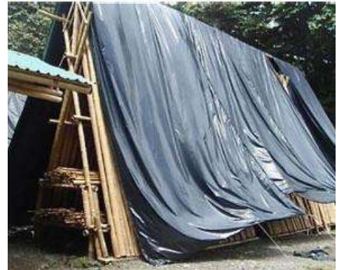
Figure 2. 48 Drying of Bamboo in the air under the tent.
