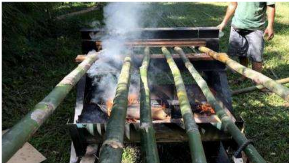
Figure 2. 44Smoke Treatment of Bamboo
