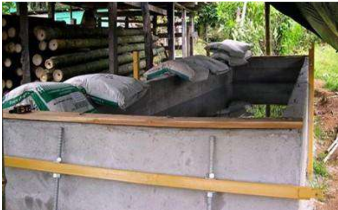
Figure 2. 45Curing of Bamboo with Borax and Boric Acid
