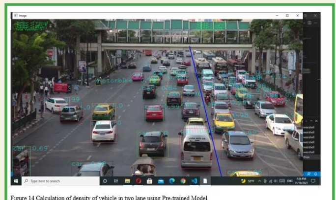
Figure 14 Calculation of density of vehicle in two lane using Pre-trained Model
