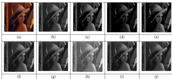
Fig 7 (a) Original image (b) Noisy Image, Denoised by: (c) VISUshrink Hard (d) VISUshrink Soft (e) VISUshrink semi-soft (f) Level Shrink Hard (g) Level Shrink Soft (h) Level Shrink semi-soft (i) SureShrink (j) Bayes Shrink
