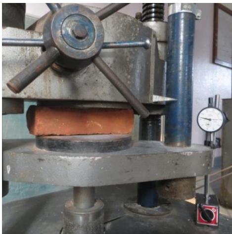
Fig. 1 Brick compression test
