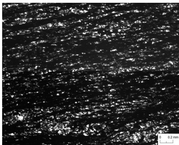
Fig 9 Photomicrograph (4x10) of the carbonaceous slate of the Benihat Slates in Bar Khola Section, showing the proportion of the carbon.
