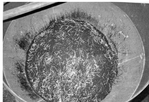
Photo 6 Condition of pre-mix (dry mix of aggregates and fibers, SF=4%, by volume)
