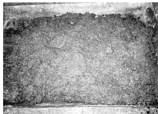
Photo 7 Mixing condition of SFRC (SF=4%, by volume)
